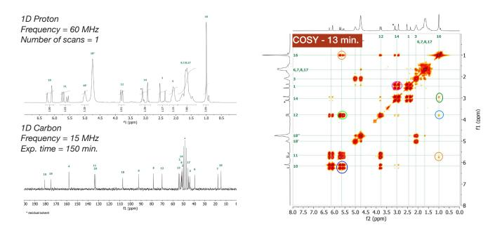
60 MHz NMR spectra of Gibberelic acid at 250 mMolar concentration
