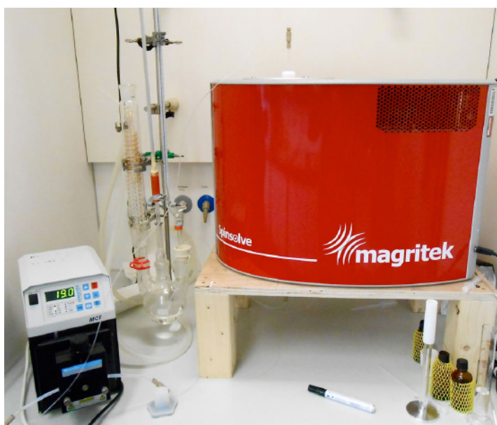
Spinsolve NMR spectrometer set up in a fume hood to monitor a batch reaction
