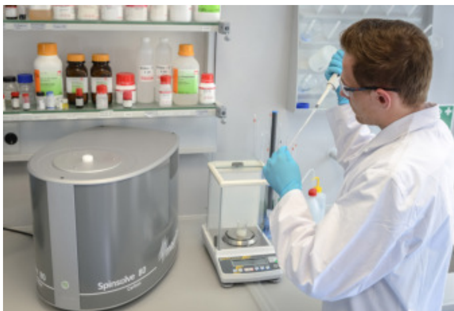
Figure 1. Spinsolve NMR spectrometer used in the chemistry lab for quick analysis of products. The typical presence of protonated solvents in the sample requires the use of solvent suppression and carbon decoupling methods to acquire the spectra of analytes of interest.
