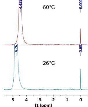
NMR Thermometer: DSS in H<sub>2</sub>O spectra acquired at different temperatures. The chemical shift differences are in excellent agreement with the calibration values of the NMR thermometer.
