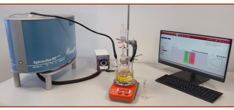
Experience the latest advancement in Spinsolve temperature control, combining unmatched stability with an effortlessly integrated heating system. Designed for precision and ease of use, this innovation ensures consistent resolution and sensitivity across the entire  $RT - 60^{\circ}C$  temperature range.
