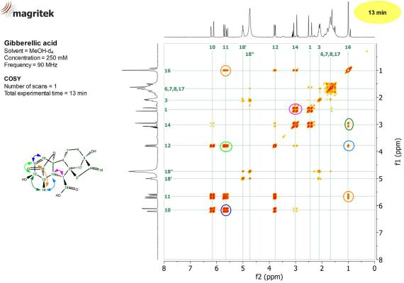
Figure 3: <sup>1</sup>H 2D COSY experiment of a 250 mM Gibberellic acid sample in MeOH-d<sub>a</sub> acquired in 13 minutes on a Spinsolve 90 MHz system.
