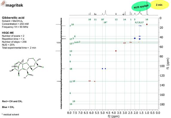
Figure 4: HSQC-ME spectrum of a 250 mM Gibberellic acid sample in MeOH-d<sub>4</sub> showing the correlation between the <sup>1</sup>H (horizontal) and <sup>13</sup>C (vertical) signals.
