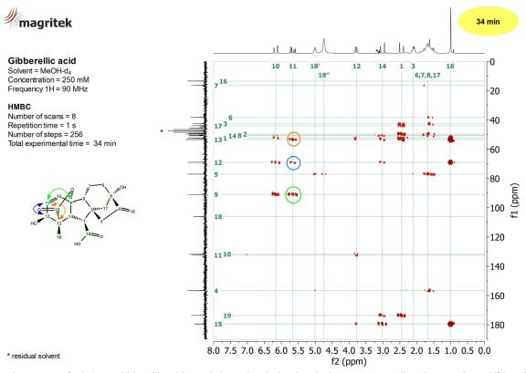
Figure 5: HMBC spectrum of a 250 mM Gibberellic acid sample in MeOH-d $_4$  showing the long-range couplings between  $^1$ H and  $^{13}$ C nuclei.
