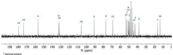
Figure 2: <sup>13</sup>C NMR spectrum of a 250 mM Gibberellic acid sample in MeOH-d<sub>4</sub> measured on a Spinsolve 90 MHz system in 60 minutes.
