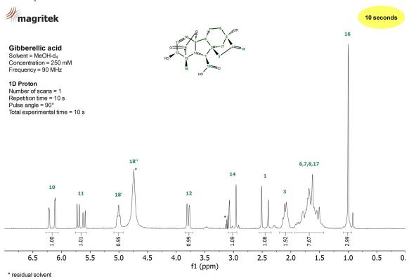
Figure 1: ¹H NMR spectrum of a 250 mM Gibberellic acid sample in MeOH-d<sub>4</sub> measured on a Spinsolve 90 MHz system in a single scan.
