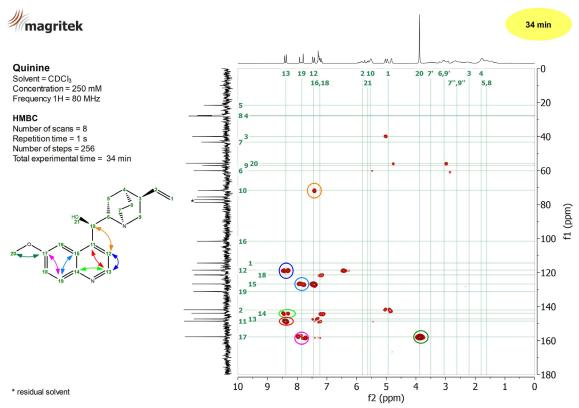
Figure 5: HMBC spectrum of a 250 mM Quinine sample in CDCl<sub>3</sub> showing the long-range couplings between <sup>1</sup>H and <sup>13</sup>C nuclei.
