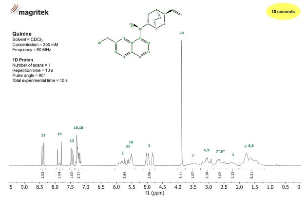
Figure 1: <sup>1</sup>H NMR spectrum of 250 mM Quinine in CDCl<sub>3</sub> measured on a Spinsolve 80 MHz system in a single scan.
