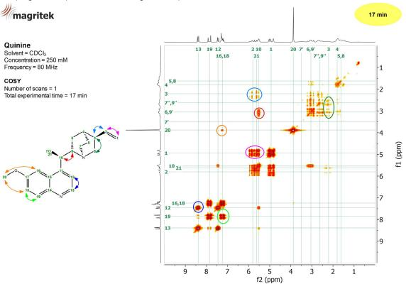
Figure 3: <sup>1</sup>H 2D COSY experiment of 250 mM Quinine in CDCl<sub>3</sub> acquired in 17 minutes on a Spinsolve 80 MHz system.
