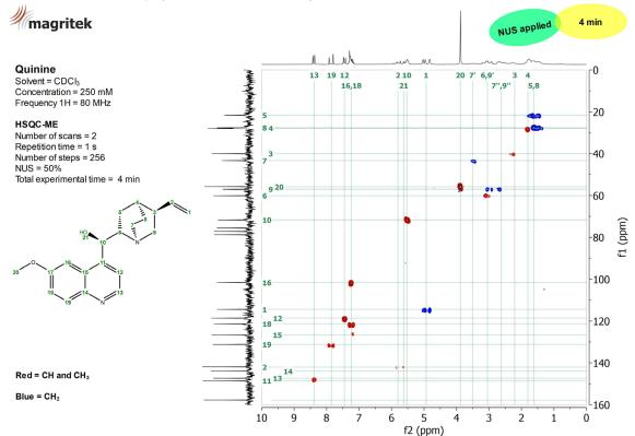
Figure 4: HSQC-ME spectrum of a 250 mM Quinine sample in CDCl<sub>3</sub> showing the correlation between the <sup>1</sup>H (horizontal) and <sup>13</sup>C (vertical) signals.
