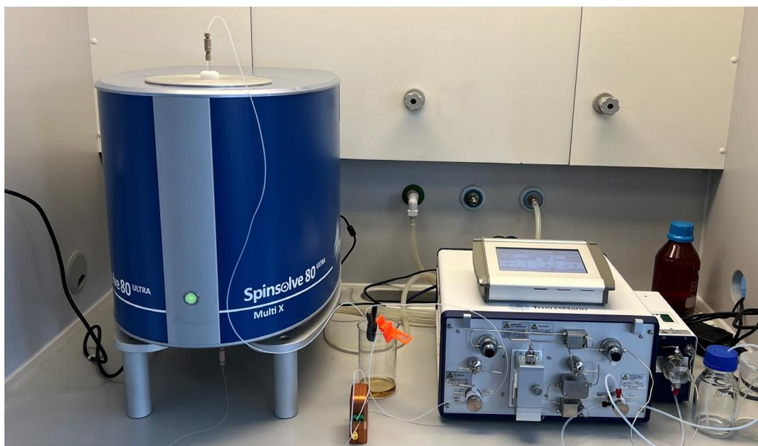
Spinsolve 80 Ultra monitoring the hydrogenation reaction performed with an H-Cube® Pro from ThalesNano.
